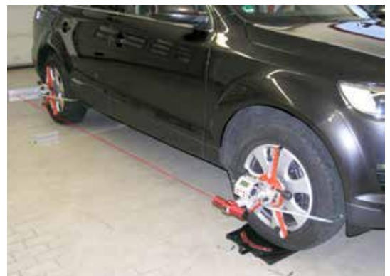
Example of a front axle measurement.
