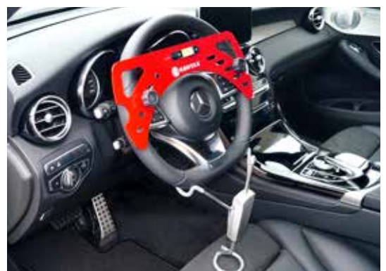
Use of the steering wheel scale and lock.
