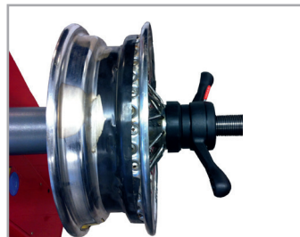
Placed spoke rim on a balancing machine. Centering is done by the center locker. The spacer keeps the distance and the cone is for the right fitting.
