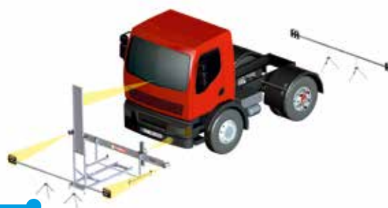
The measuring crosshead and calibration reflector are aligned horizontally at an exact distance in front of the vehicle.
